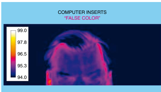
FIGURE 7.10 The final step in the sequence is the introduction of false color . This is called false color because wavelengths in this frequency have no color. The computer injects the color to make it easier for human interpretation of the image. This is an image of a "normal forehead." (see color plate)
